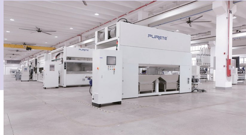
• Reciprocating spraying production line It can be UV- and water-based, and can achieve various processing techniques to meet customization needs
