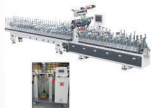
2 PUR热熔胶包覆机 Pur hot glue profile wrapping machine
